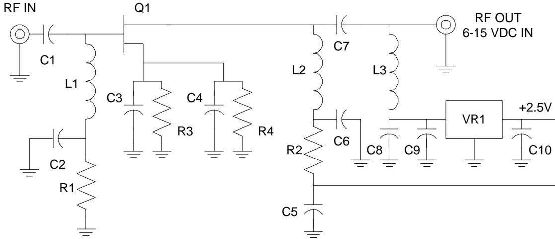
Figure 4: LNA schematic.
